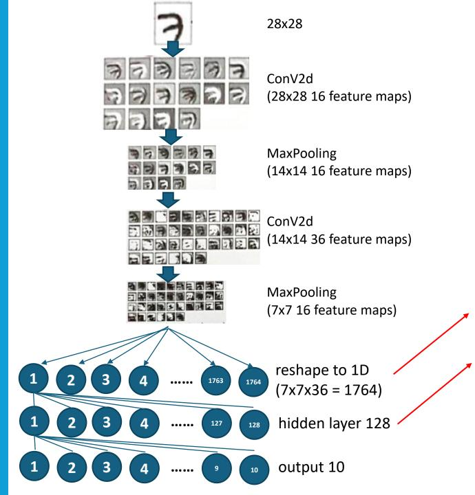
**Flattening**: Before passing the output of the convolutional and pooling layers to the FC layers, the feature maps are flattened into a one-dimensional vector. This flattening operation converts the spatial information into a linear representation.
